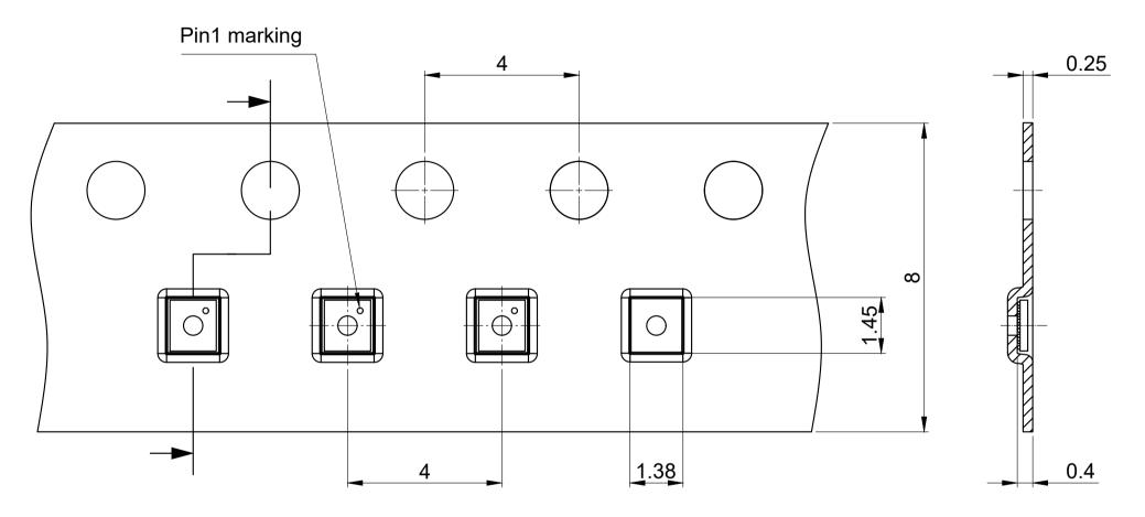
All dimensions are in units mm The drawing is in compliance with ISO 128-30, Projection Method 1 [ $\bigcirc \phi$ ]
