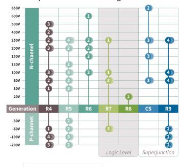
N-Channel: 20 V to 650 V P-Channel: -30 V to -200 V
