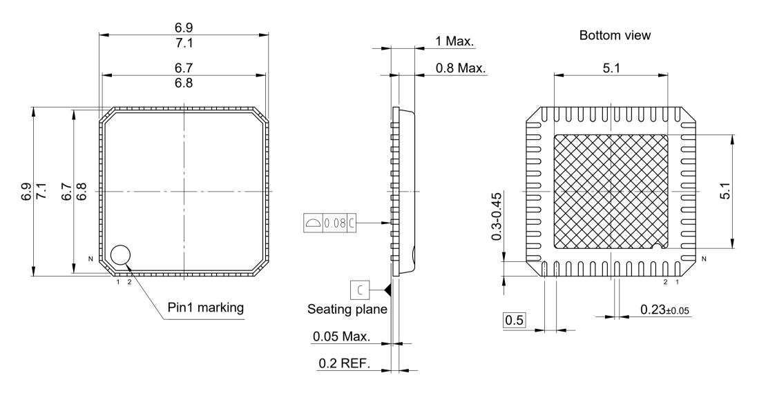
$\boxtimes$  Hatch area is solderable exposed metal.
