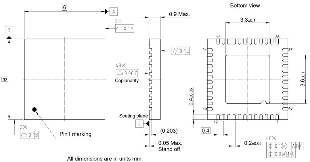
The drawing is in compliance with ISO 128-30, Projection Method 1 [ $\bigcirc \oplus$ ] Drawing according to ISO 8015, general tolerances ISO 2768-mK
