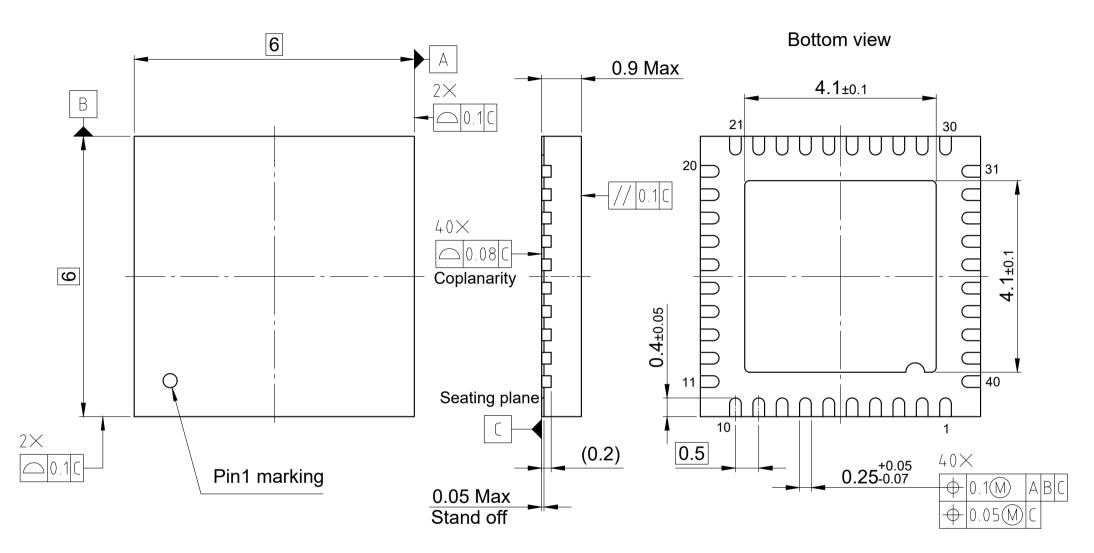
All dimensions are in units mm The drawing is in compliance with ISO 128-30, Projection Method 1 [
