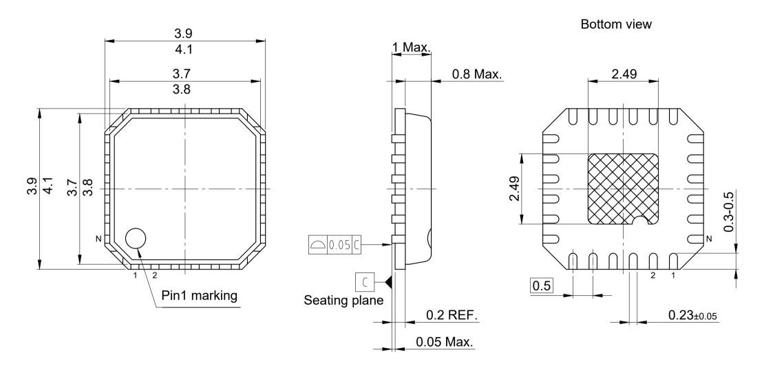
$\boxtimes$  Hatch is solderable exposed metal.
