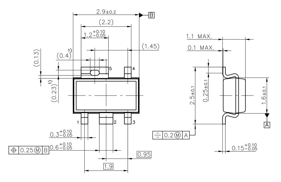
NOTE: MOLD FLASH, PROTRUSIONS OR GATE BURRS OF 0.2 MM MAXIMUM PER SIDE ARE NOT INCLUDED 1) CONTOUR OF SLOT DEPENDS ON PROFILE OF GULL—WING LEAD FORM
