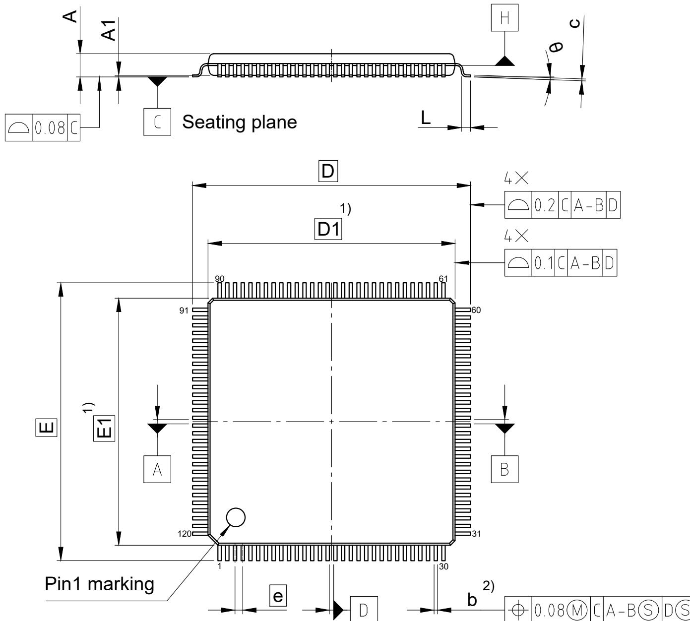
1) Dimensions D1 and E1 do not include mold protrusion. allowable protrusion is 0.25mm per side.
