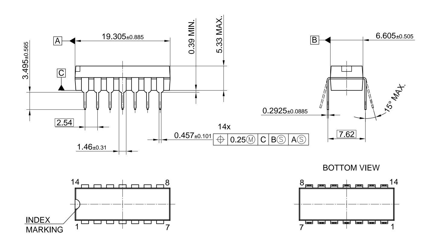
1) DIMENSION DOES NOT INCLUDE MOLD PROTRUSIONS, MOLD PROTRUSIONS SHALL NOT EXCEED 0.25 ALL DIMENSIONS ARE IN UNITS MM THE DRAWING IS IN COMPLIANCE WITH ISO 128 & PROJECTION METHOD 1 [ $\bigcirc$  $\bigcirc$ ]
