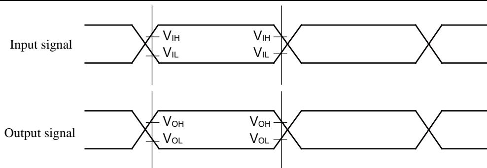
**Separate Bus Access Asynchronous SRAM Mode**
