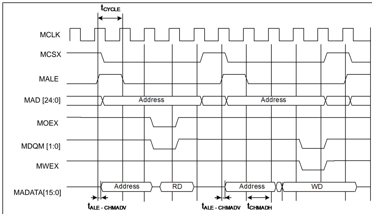
**Multiplexed Bus Access Synchronous SRAM Mode**
