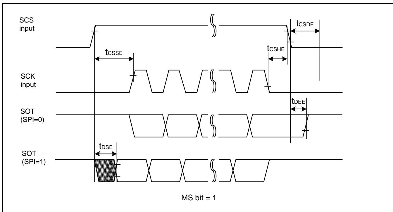
**External Clock (EXT = 1): when in Asynchronous Mode Only**
