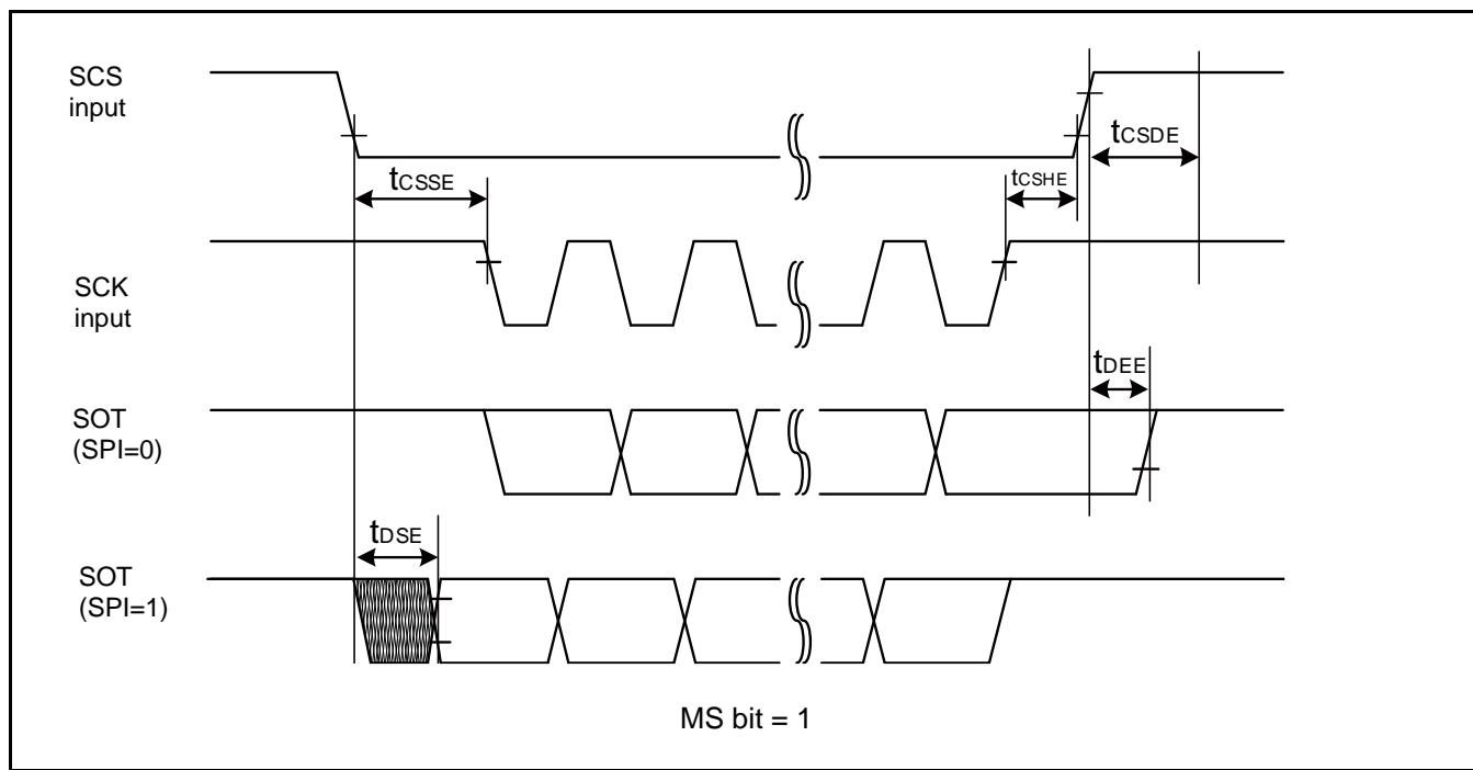
**When Using High-Speed Synchronous Serial Chip Select (SCINV = 1, CSLVL=1)**
