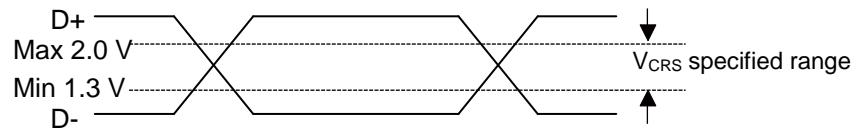
\*5: They indicate Rising time ( $t_{FR}$ ) and Falling time ( $t_{FF}$ ) of the Full-speed differential data signal.
