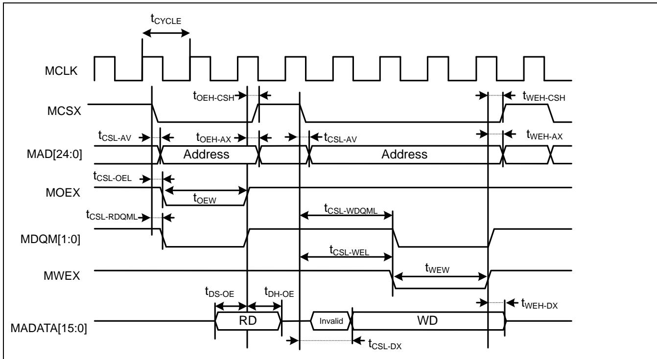
**Separate Bus Access Synchronous SRAM Mode**
