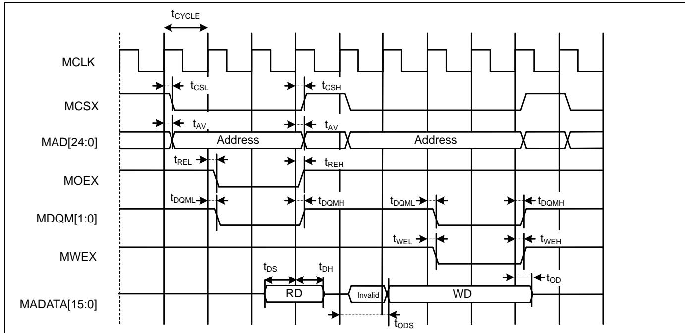
**Multiplexed Bus Access Asynchronous SRAM Mode**
