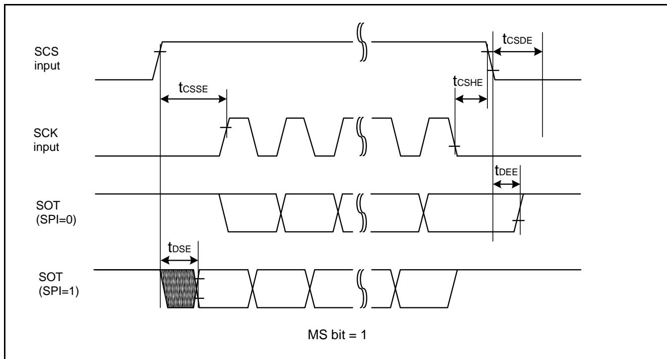
**High-Speed Synchronous Serial (SPI = 0, SCINV = 0)**
