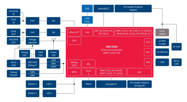
The block diagram shows the main components of the XMC4800 IoT Amazon FreeRTOS connectivity kit WiFi and their interconnections.
