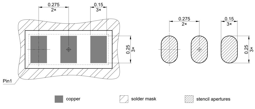
Based on stencil thickness 0.06 All undimensioned radii are 0.075 All dimensions are in units mm
