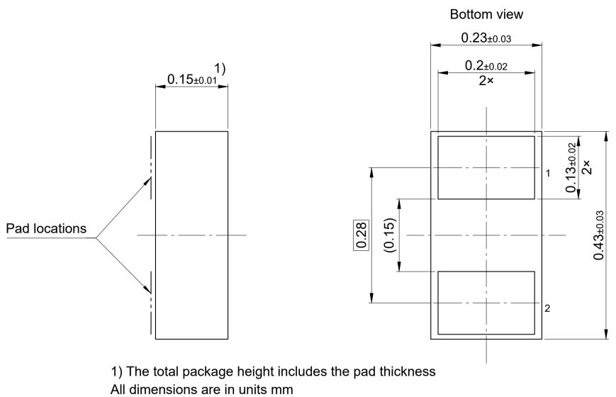
The drawing is in compliance with ISO 128-30, Projection Method 1 [ $\bigcirc \phi$ ] Drawing according to ISO 8015, general tolerances ISO 2768-mk
