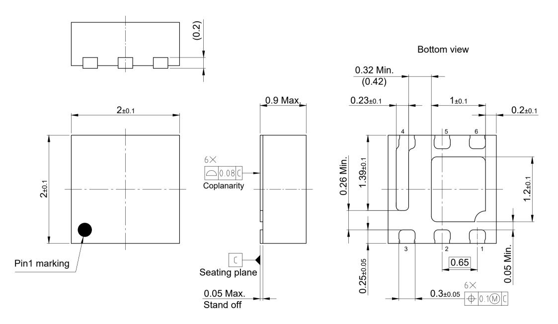
All dimensions do not include mold flash or protrusion.
