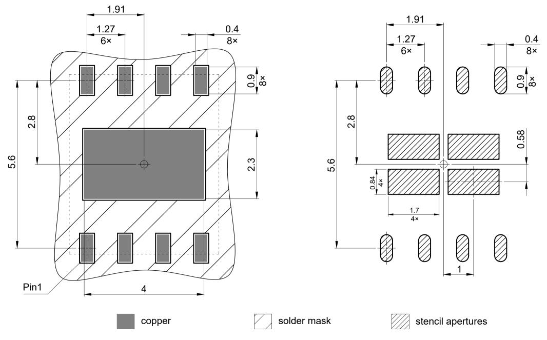
All pads are non-solder mask defined All undimensioned radii are 0.2 All dimensions are in units mm
