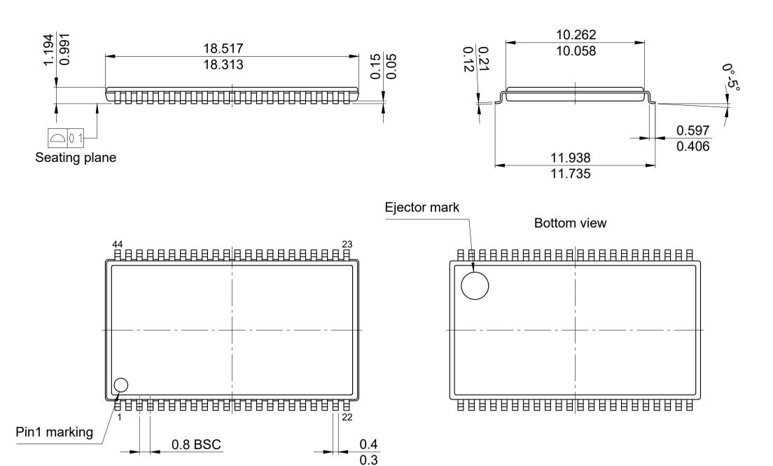
All dimensions are in units mm  $\frac{\text{max.}}{\text{min.}}$ The drawing is in compliance with ISO 128-30, Projection Method 1 [
