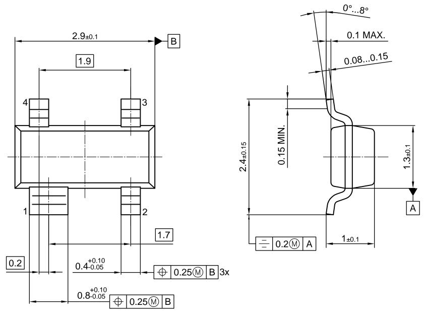
MOLD FLASH, PROTUSIONS OR GATE BURRS OF 0.2MM MAXIMUM PER SIDE ARE NOT INCLUDED ALL DIMENSIONS ARE IN UNITS MM THE DRAWING IS IN COMPLIANCE WITH ISO 128 & PROJECTION METHOD 1 [  $\bigcirc$   $\bigcirc$
