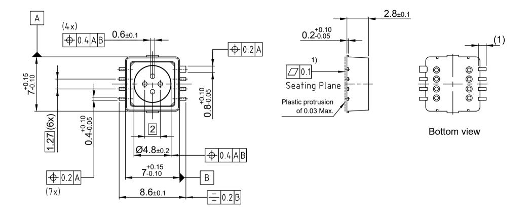
Outer dimensions does not include protrusion or intrusion of 0.2max. per side
